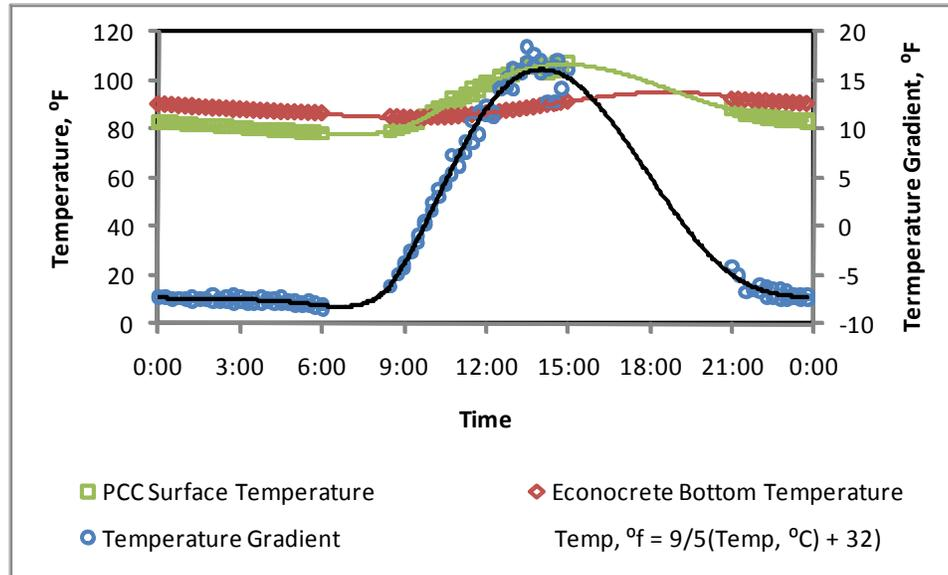
**FIGURE 7 Concrete temperature measurements.**
