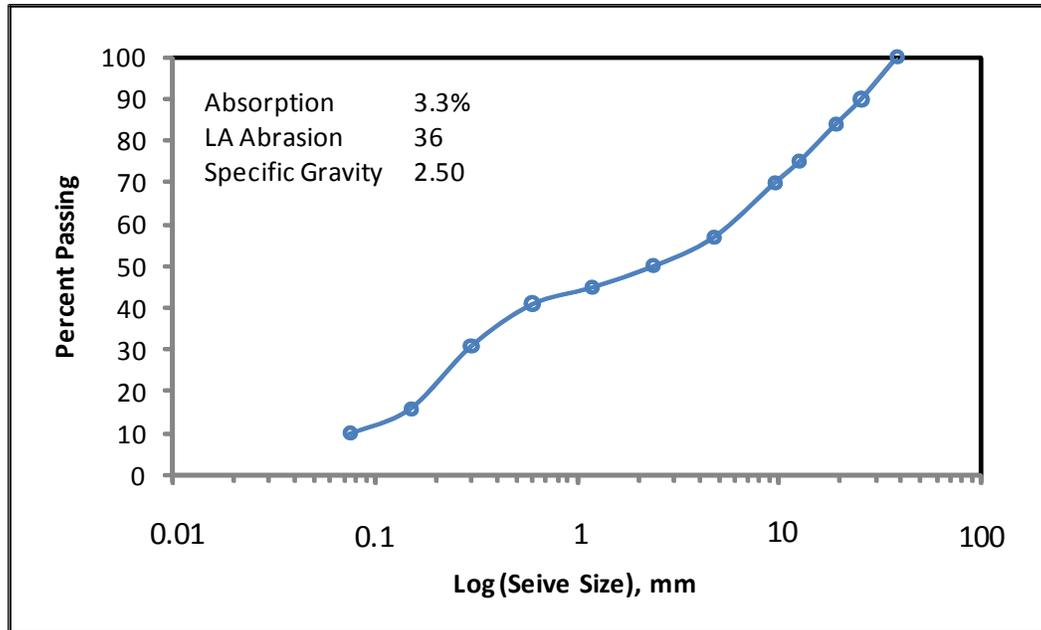
**FIGURE 4 Econcrete aggregate properties.**
