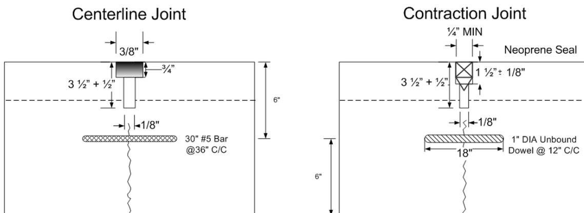
Note: Dowel bars specified for sections 3A and 3B only.
