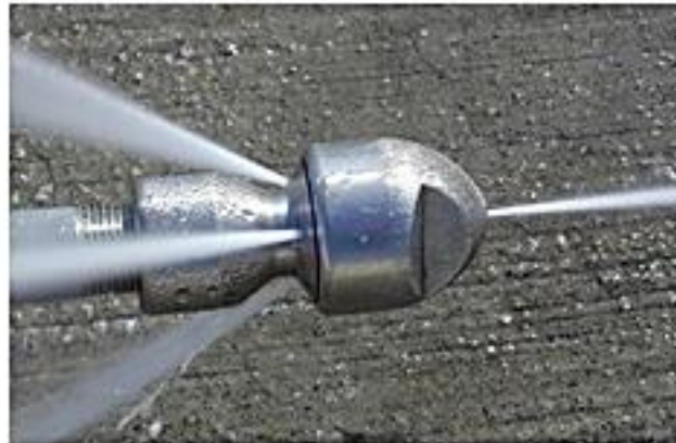
Forward Jet nozzles used for cleaning clogged pipes
