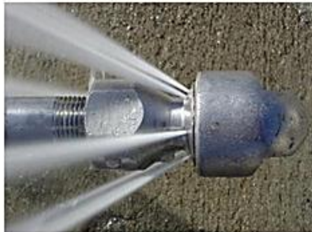
Rear Jet nozzles used for cleaning pipes that are not clogged
