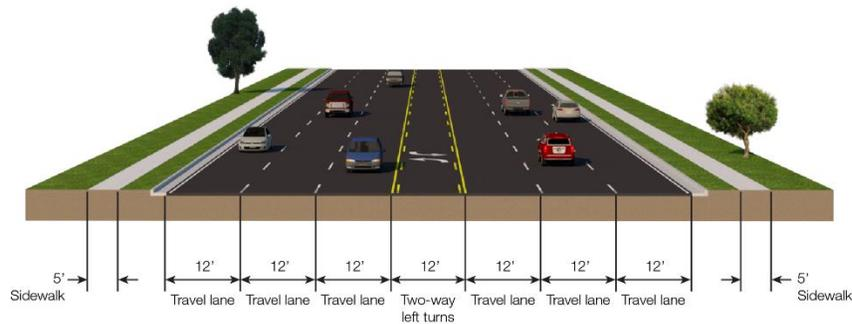
Figure 5. Typical Six-Lane with Center Turn Lane Roadway Section for Parallel Corridors
