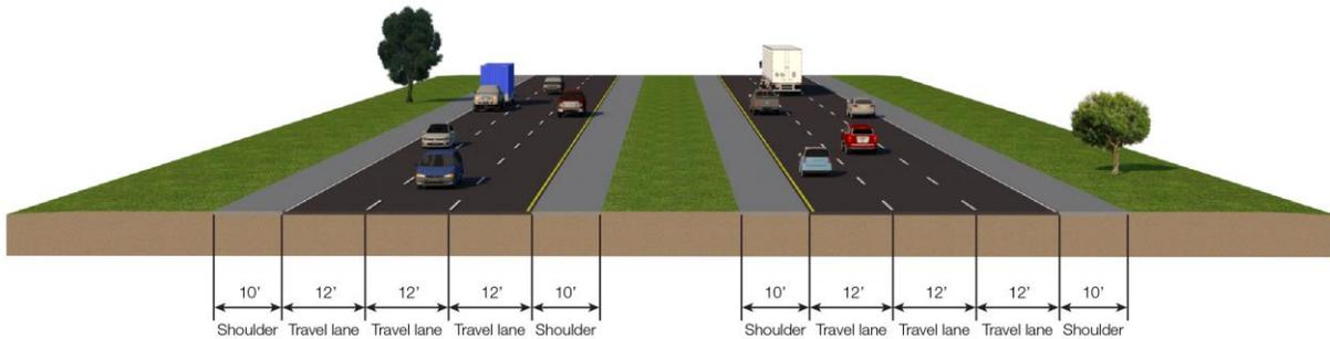
Figure 3. I-75 Roadway Typical Section
