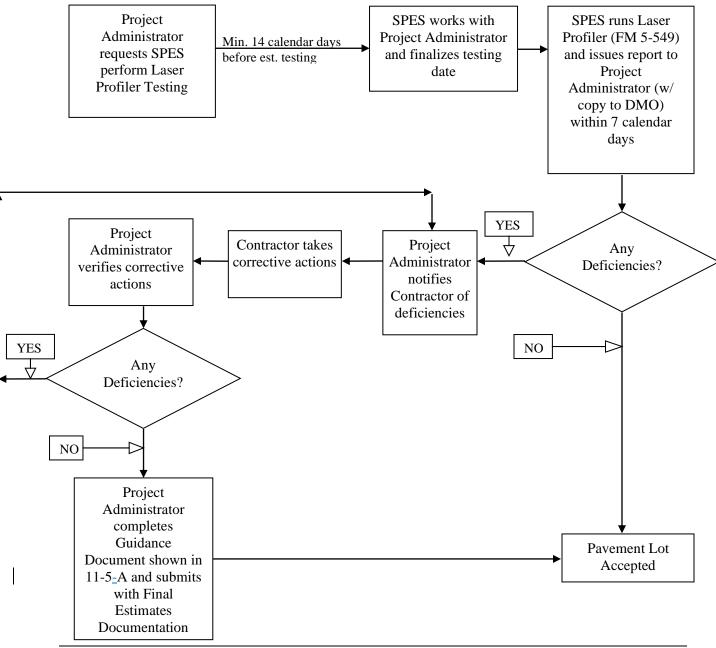
Testing and Correcting Asphalt Pavement Surface Deficiencies
