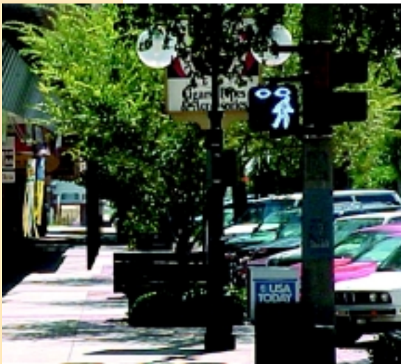
A scanning eyes pedestrian signal head at a crosswalk along Central Ave in downtown St. Petersburg, Florida.
